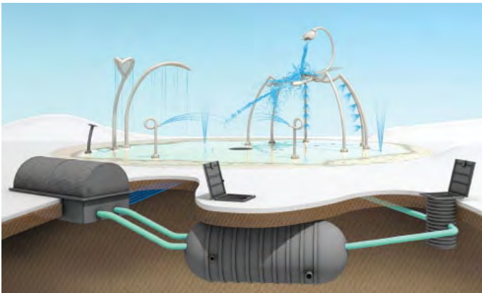
Figure 2.25: Recirculating Splash Pad (Source: PlayQuest)
